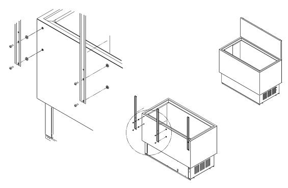
Attach the display sign's mounting brackets to the back of the case using pre-drilled holes. Insert the washers between the brackets and the case. Fasten screws.
