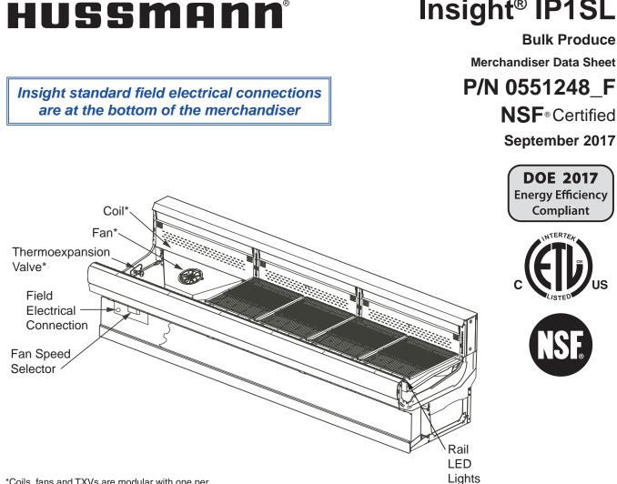
\*Coils, fans and TXVs are modular with one per 3 or 4 foot section.
