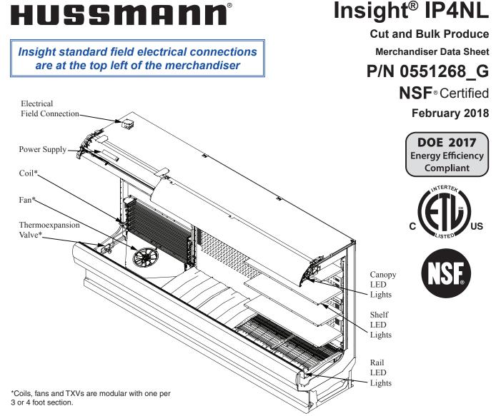
Portion of parts removed for clarity.
