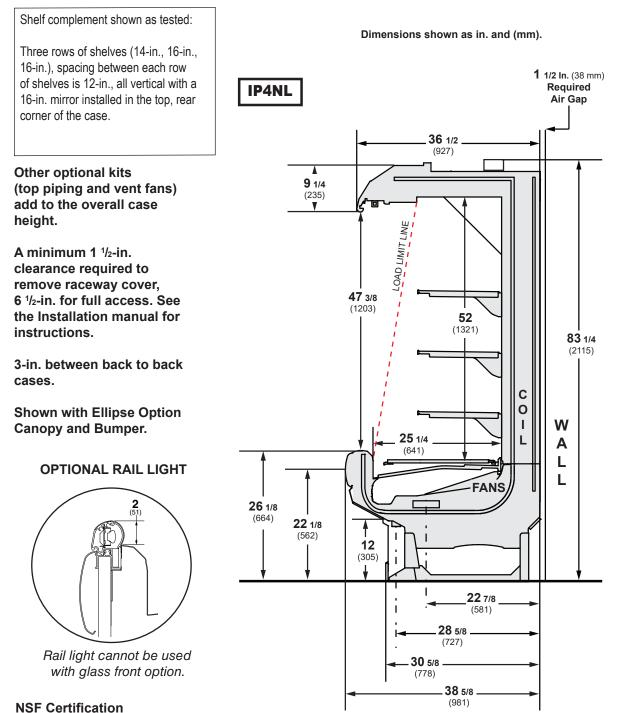
This merchandiser model is manufactured to meet NSF/ANSI (National Sanitation Foundation) Standard #7 requirements for construction, materials and cleanability.
