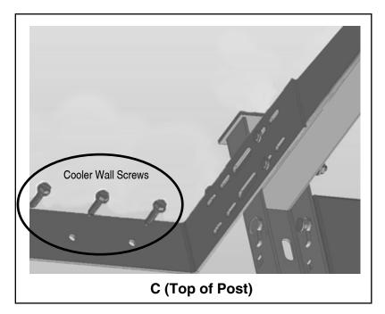
4 Assemble the Center Kit similar to Step 2 and attach to End Kit. Continue installing Center Kits for the remaining length of the doors. Ensure shelf kits are level - adjust levelers if needed.
