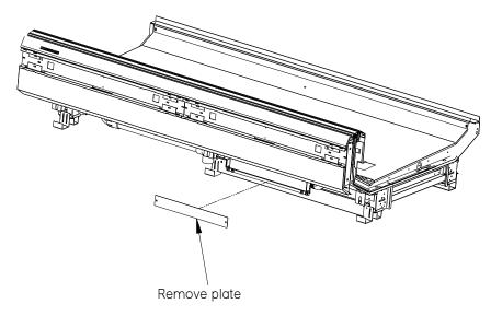
4. Remove Plate to access Controller Service Box.
