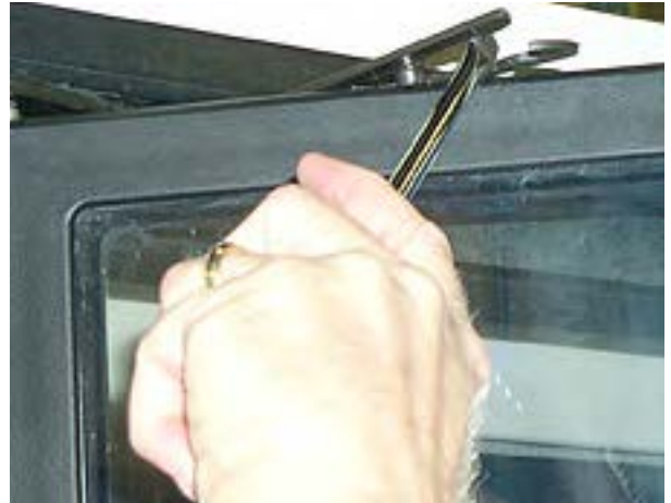
Lift Door Retainer Over Shoulder Screw
