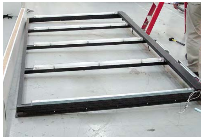
Unpack Frame and Lay Face Down
