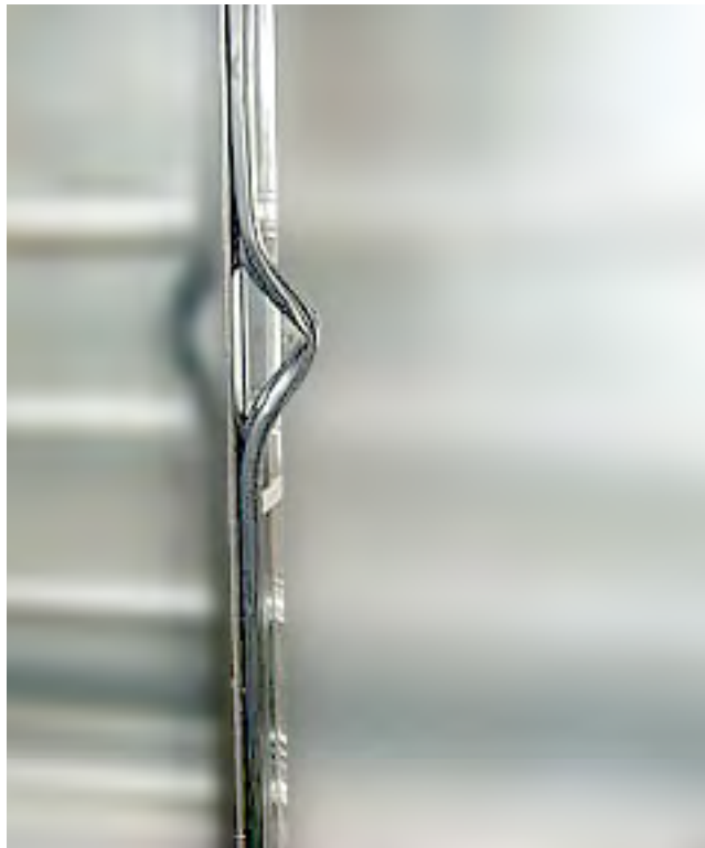
Improperly Installed or Damaged Gasket
