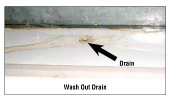
The washout drain flows into an auxiliary waste line. Next, remove the auxiliary waste line cap to drain any excess water. Place a dry towel over the line to absorb water.
