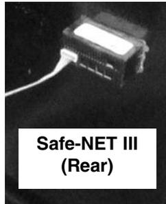
Be careful not to detach Safe-NET III cable from display when removing access panel.
