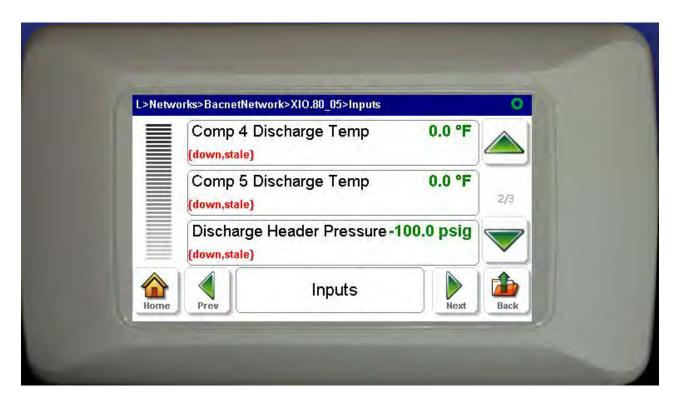
You can scroll up or down to view the sensor readings. NOTE: In this example, the communication network is down, so sensor readings would not be true. You can only trust the readings when communications is healthy.
