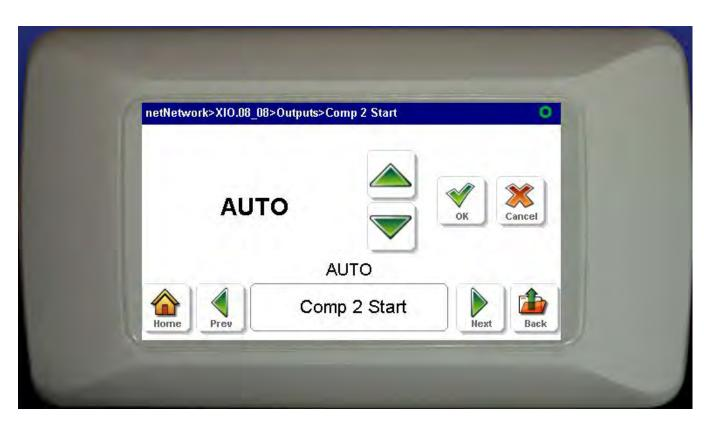
To override an output, you must first enter an access code. Contact Walmart for the access code. After entering the code, use the up and down arrow keys to force the output on, or off, or to return it to Automatic operation. If you are overridding a modulating output, you can use the up/down arrow keys to force the 0-10V output to the desired control voltage. **NOTE:** When done, return all outputs to Auto.
