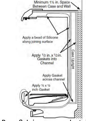
Prep & Join case per Installation Manual once case is **POSITIONED & LEVELED.**
