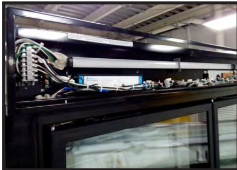
LED and Power Supply Shown with Display Panel Removed
