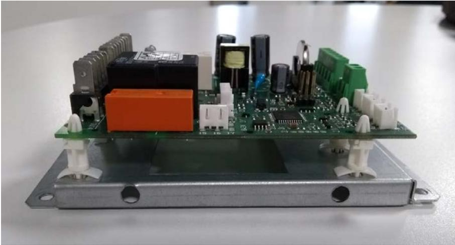
6. Use the Hex Head 5/16" screw to secure the assembly inside the control box.
