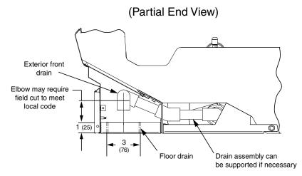
**IMPORTANT:** If hub drain is used in lieu of flush floor sink, a drain extension kit must be installed. Hub drains must be located in front of the waste outlet to achieve adequate air gap.
