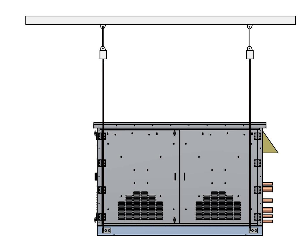
1. MAXIMUM SHIPPING WIDTH OF UNIT, INCLUDING STUB OUT: 102.00". 2. IN CASE OF CONDENSER MOTOR CHANGE UNIT HEIGHT AND WEIGHT WILL VARY. 3. 20X36 RECEIVER WILL BE MOUNTED INSIDE THE UNIT, IN CASE OF RECEIVER OTHER THEN 20X36 SIZE, IT WILL BE MOUNTED UNDERNEATH THE CONDENSER.
