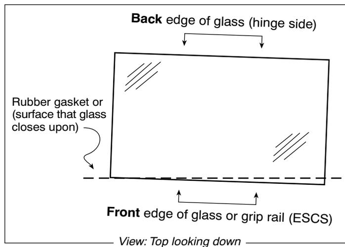
A glass panel that does not close smoothly and neatly, most likely is misaligned with the front edge of the glass and the surface or edge which it closes upon. Refer to diagram above. To correct problem Go to Item 5.
