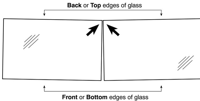
B. If pinched at the bottom: Gap is more narrow at the bottom than at the top. Then see Item 4 / Uneven Gap
