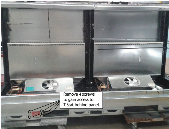
Step 1: Removal of cover: With power off remove screws and pull cover off
