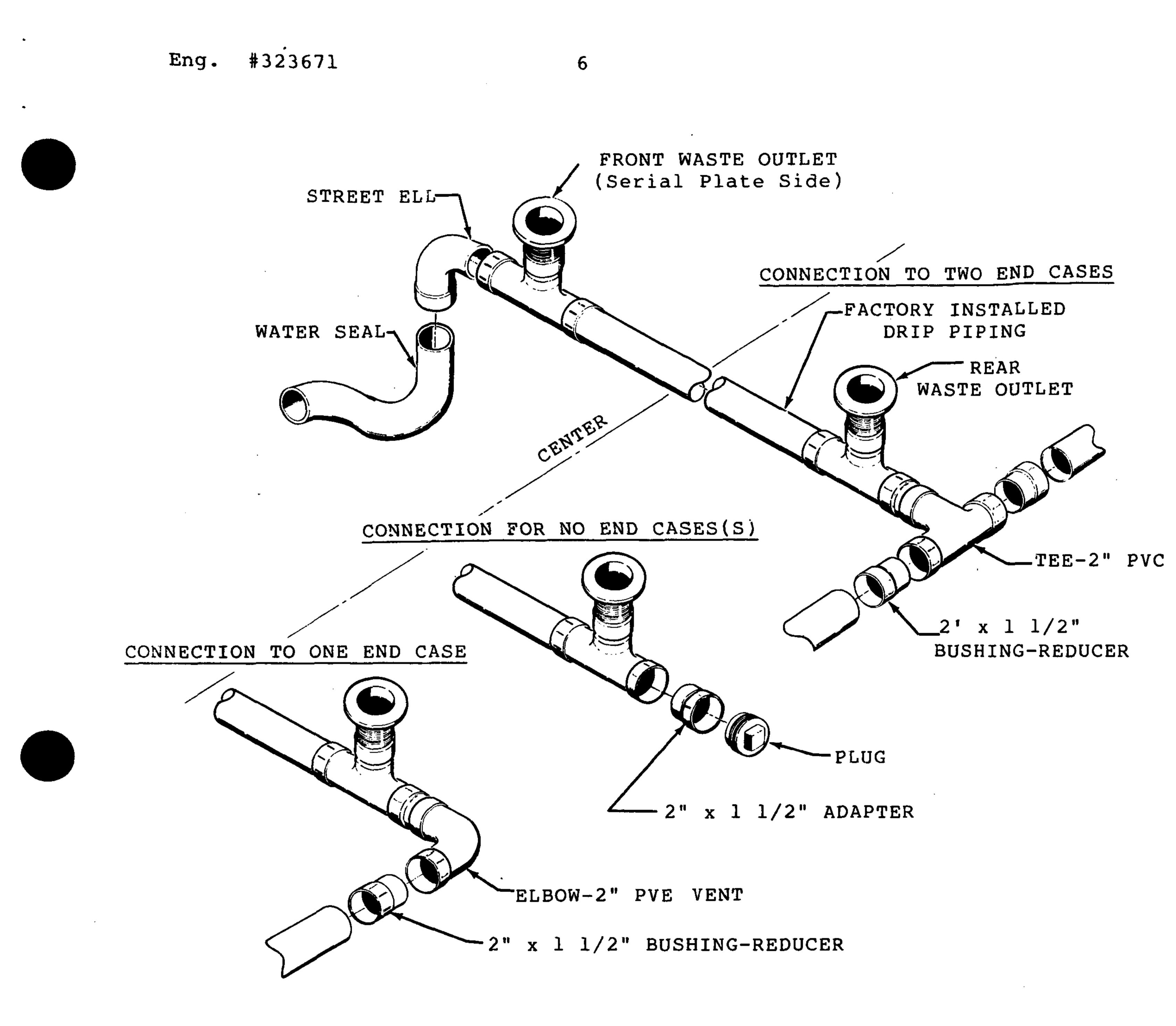
When a 6' end case is joined to one end of both ends of the parent case, all interconnecting piping of the six foot end case will be complete and the water seal can only be installed to the front of the case as shown above.
