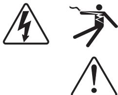
The addition of either symbol to a “Danger” or “Warning” safety label indicates that an electrical hazard exists which will result in personal injury if the instructions are not followed.
