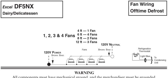
All components must have mechanical ground, and the merchandiser must be grounded. CIRCLED NUMBERS = PARTS LIST ITEM NUMBERS
