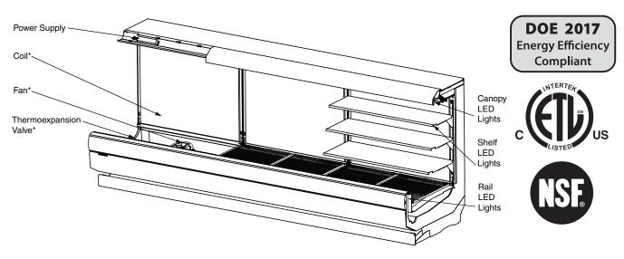
\*Coils, fans and TXVs are modular with one per 3 or 4 foot section.
