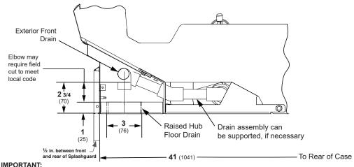
DRAIN EXTENSION KIT REQUIRED TO PIPE MULTIPLE CASES TO ONE DRAIN OR TO USE A RAISED HUB DRAIN
