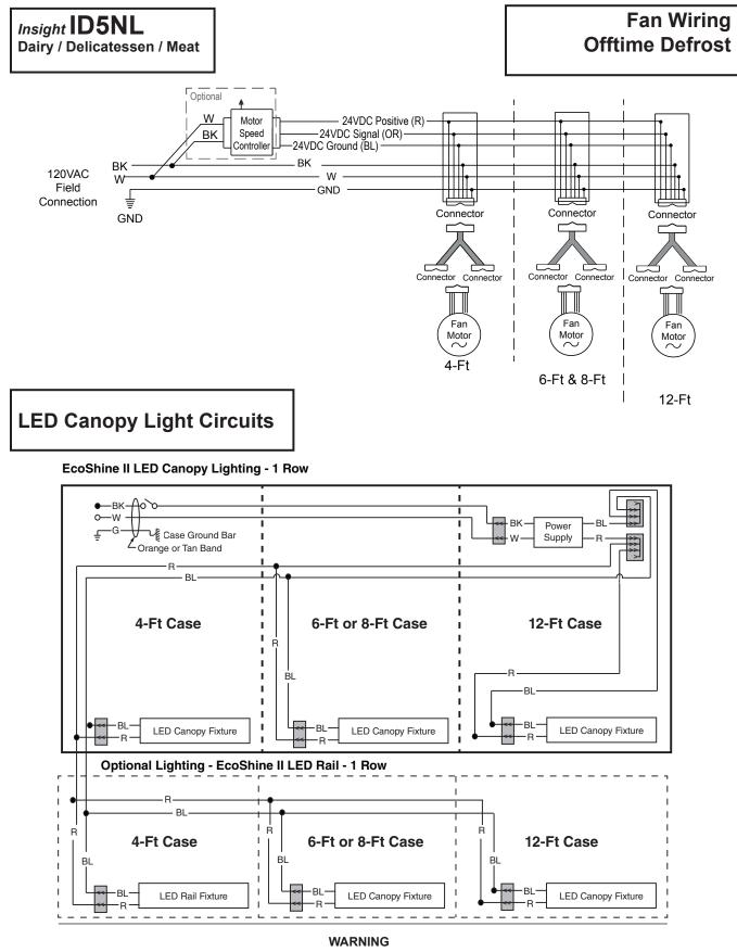
All components must have mechanical ground, and the merchandiser must be grounded.
