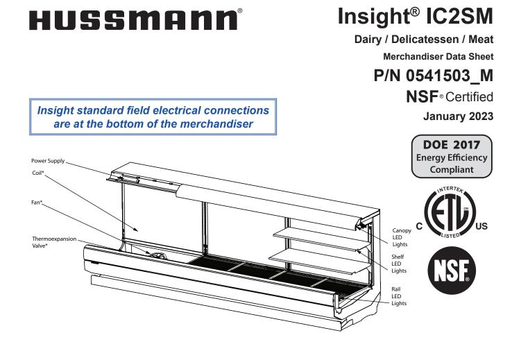
\*Coils, fans and TXVs are modular with one per 3 or 4 foot section.
