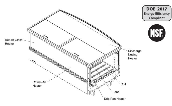
Note: Portion of parts removed for clarity.
