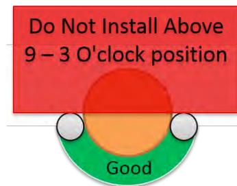
Incorrect position of sensor can result in reduced performance.
