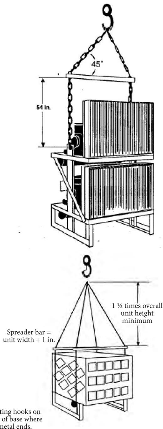
Figure 1-1 Rigging and Lifting
