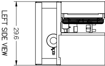
MAIN ELECTRICAL CONNECTION BEHIND CONTROL PANEL
