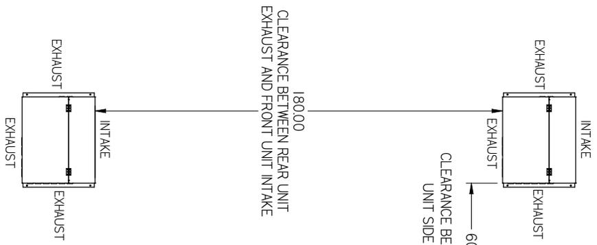
**CLEARANCE BETWEEN MULTIPLE UNIT SIDE EXHAUSTS**
