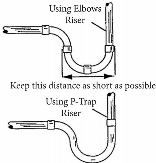
Figure 3-4 P-Trap Construction
