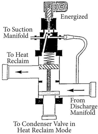
Figure 2-8 Heat Reclaim Valve Heat Reclaim Mode
