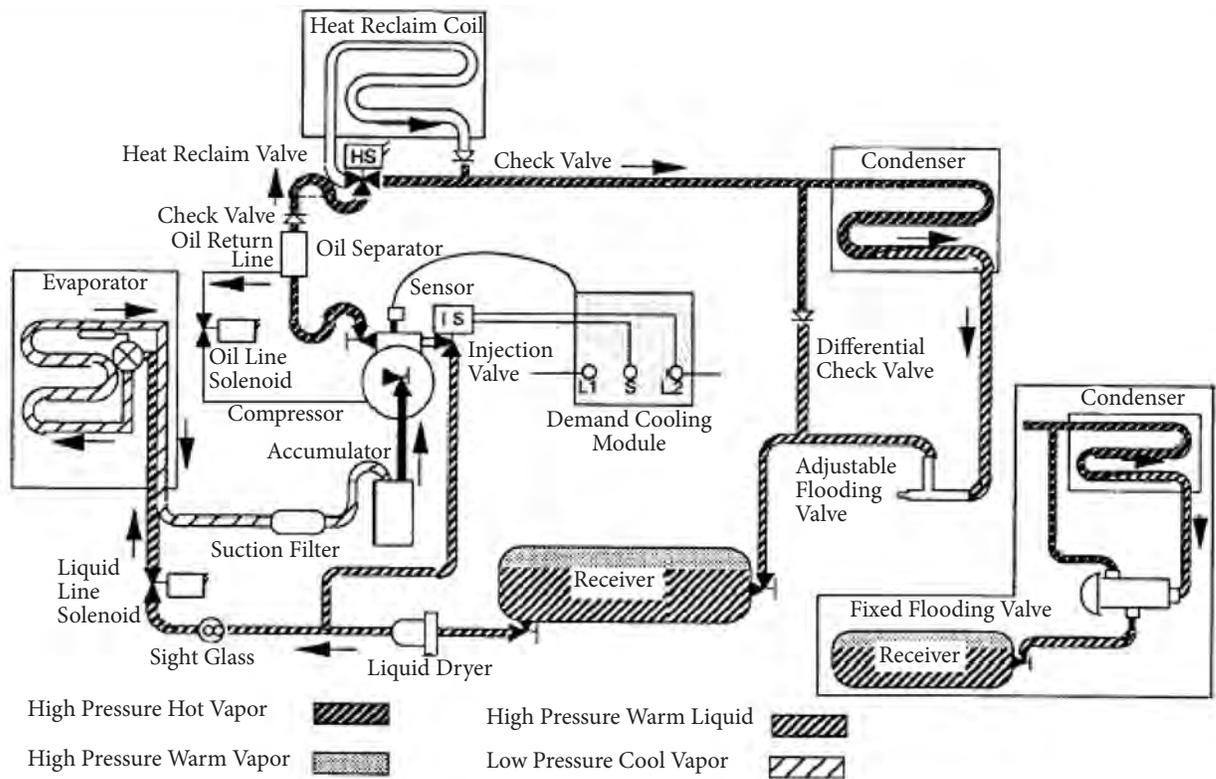
Figure 2-1 Refrigeration Cycle
