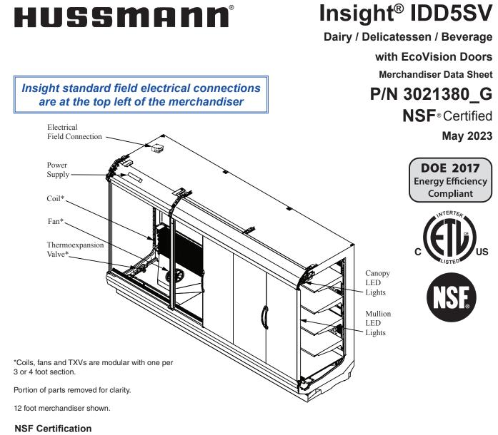
This merchandiser model is manufactured to meet NSF/ANSI (National Sanitation Foundation) Standard #7 requirements for construction, materials and cleanability.
