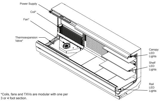
Portion of parts removed for clarity.
