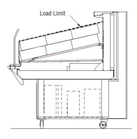
Q2SSM4S & Q2SSM6S Load Limit Line
