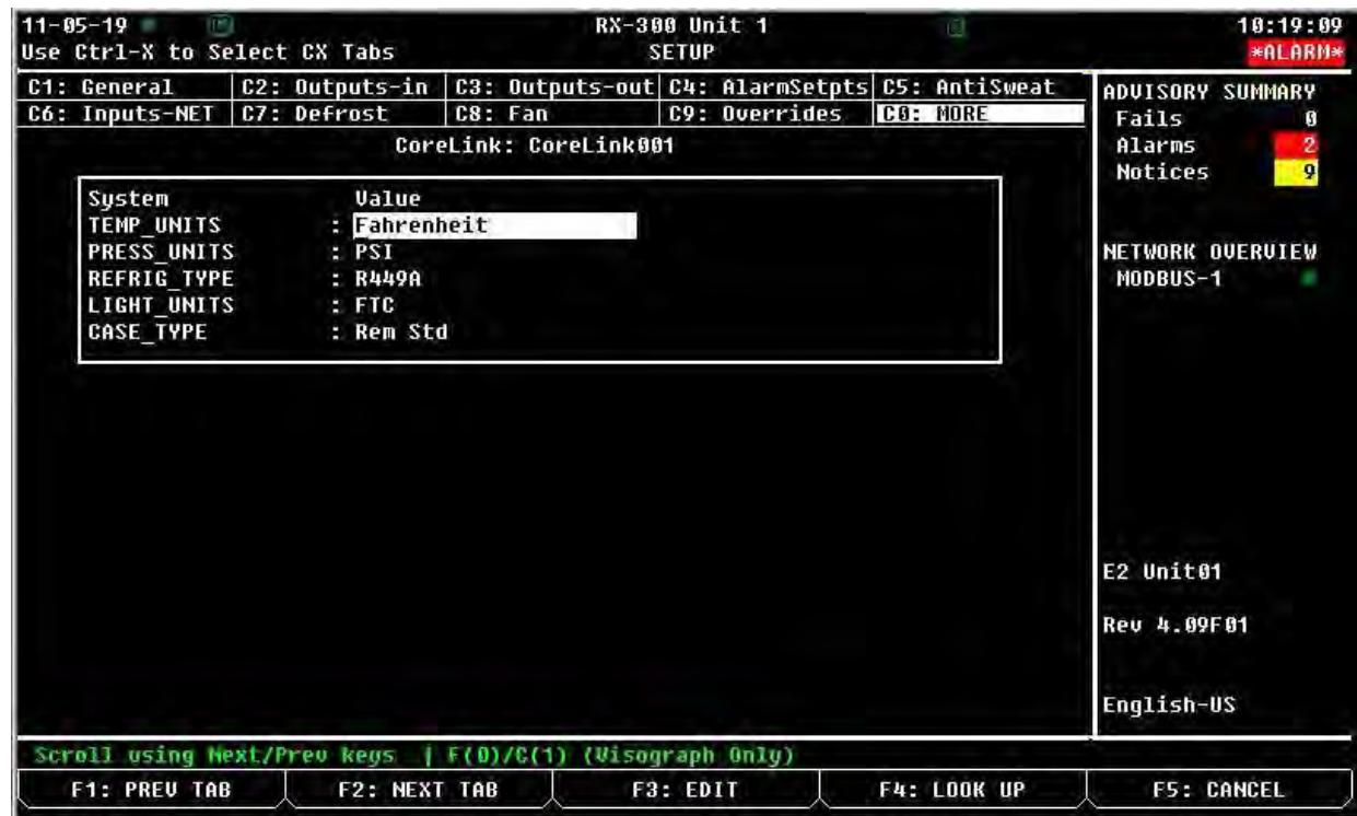
Navigate to C0: More and then to System Data to check 5 Read/Write description of temp, pressure & Refrigerant and case type as below. Check for correct data. If not press F3 to edit parameter list
