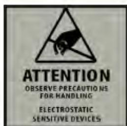
Hussmann recommends industry workers use antistatic wrist straps, ESD wrist strap, or ground bracelet when working on electronic devices which can be damaged by ESD. Please consult chosen strap literature for best practices for usage.
