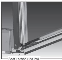
Seat Torsion Rod into plate assembly. Rotate door slightly to verify torsion rod is seated properly.
