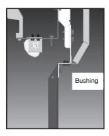
8. Install the bottom plate assembly in the Support Rail. The bottom plate assembly is marked "L" and "R". Frame of reference is standing in front of the case. Repeat for other openings.
