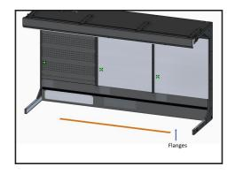
Place Bottom Support over Support Rail and center with the bottom uprights on case.
