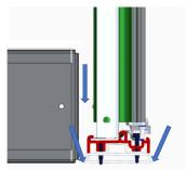
Seal the inside and outside of Support where it meets the floor. Seal any gaps between the end uprights. 1-22
