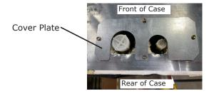
2. Pull up the inlet/outlet lines to same height as the condensing unit refrigeration lines. Ensure refrigeration lines are centered in the cutout.
