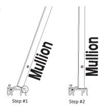
Slide top flange on mullion through slot in canopy support. Attach with screw. Repeat for all center and end mullions.
