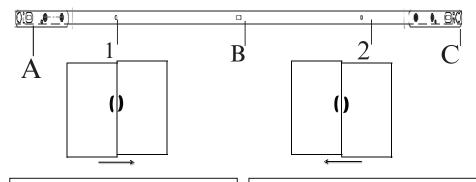
To Correct Shift the Bottom Plate to the Right
