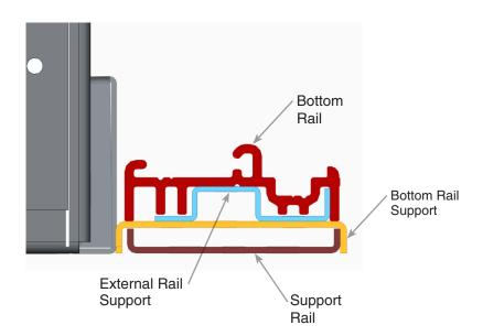
5. Install mullions onto Support Rail. Angle the mullion toward inside of the case and engage the flange in the extrusion (Step 1). Straighten mullion (Step 2).
