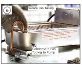
Condensate Pan (Installed on top of case)
