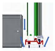
Seal the inside and outside of Support where it meets the floor. Seal any gaps between the end uprights.
