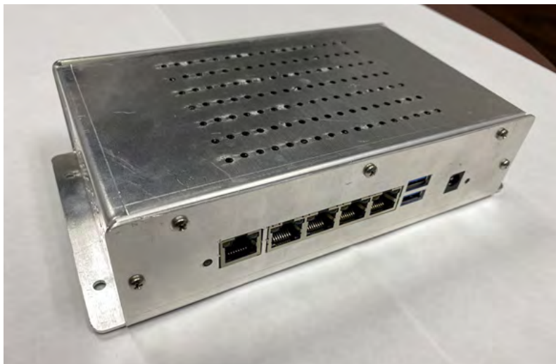
Figure 1: Case front and bottom with mounting tabs shown
