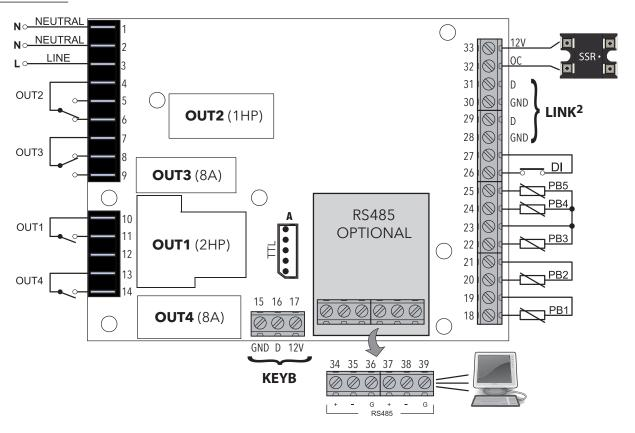
\* N.B.: analogue inputs PB1...PB5 can also be configured as Digital Inputs DI.
