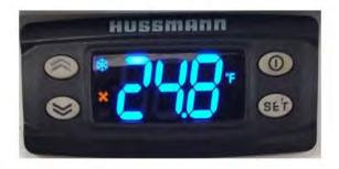
This cabinet temperature may reflect the refrigeration cycle of the Set-Point and its' Differential. The most accurate temperature on a cabinets operation is to verify the product temperature.
