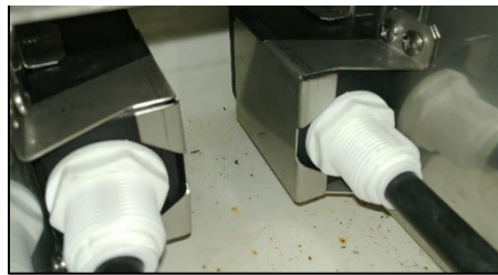
Figure 5: Pre-installed brackets shown with nozzles installed. The required bracketry will be factory installed.
