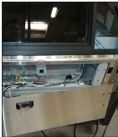
Figure 15: The system clock interrupts the fogging system during non-display hours.
