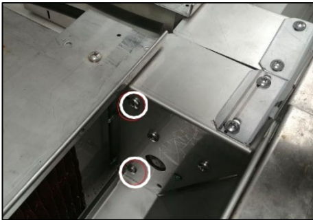
Figure 6: Remove indicated screws and remove close off and mount nozzles.
