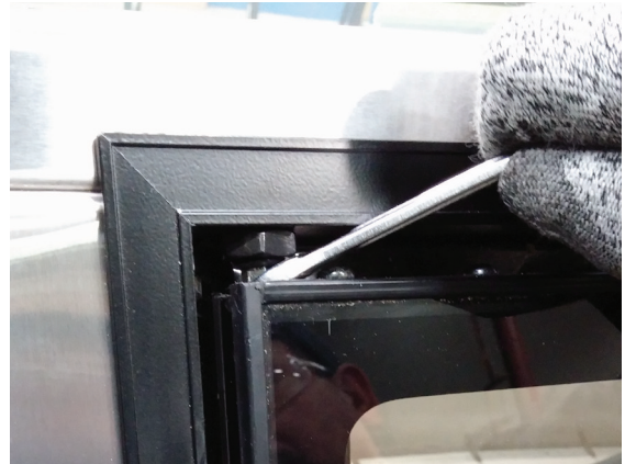
Figure 1. Turn and hold the top hinge pin
