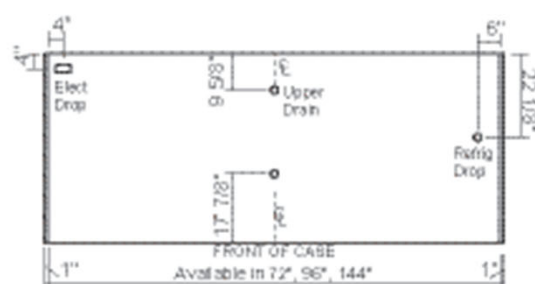
R3HV CR3HV R3HV-F CR3HV-F R3HV-M CR3HV-M Service Cases with Self Service Front Plan View Scale = 1/4"
