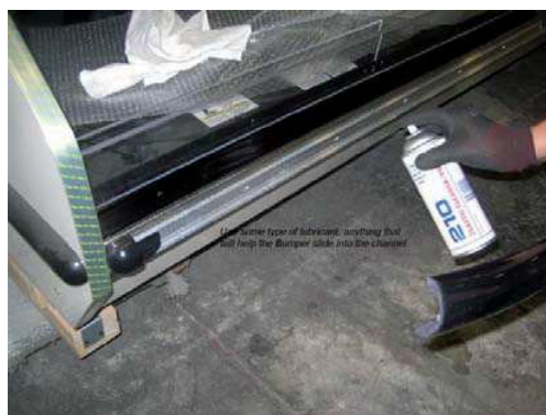
Step 2: Use silicone lubricant to help the bumper slide into the channel.
