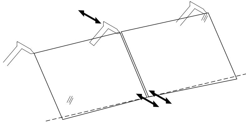
B. Adjust outside hinges (Center hinge stationary) As this diagram indicates, pulling the outside hinge further back, pulls the outside edge closer to the surface or edge which the glass rests upon. And pushing the middle hinge to the front, pushes the inside edges further away from the surface or edge which the glass rests upon.
