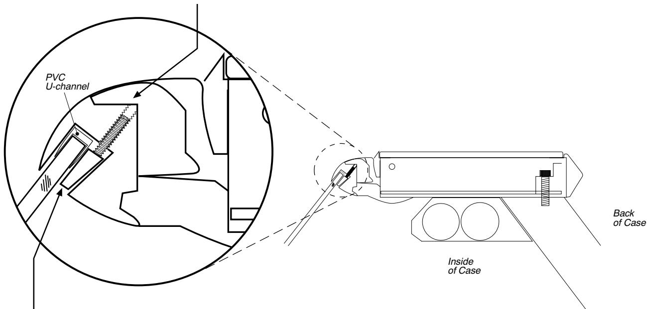
3. Use tip of screwdriver to gently tap loose wedge the entire length of the panel
