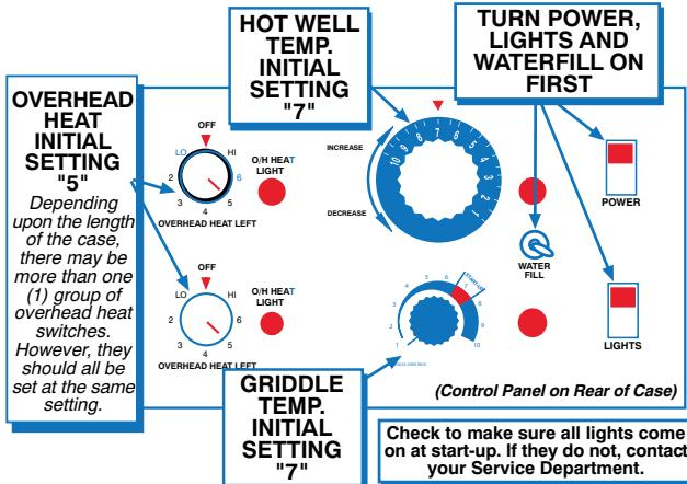
5. Place empty pans in the case to help the case preheat faster. The unit will take approximately 45 minutes to preheat. It is also important that the small pan divider bars are installed properly between each pan. These dividers provide a seal around each individual pan and are necessary to maintain the proper temperature of the food products. Extra dividers should be stored outside of the case.
