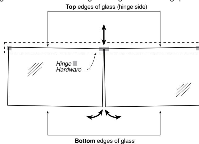
B. Adjust outside hinges (Center hinge stationary) This diagram indicates that raising the outside hinges widens the gap at the bottom; whereas, lowering the outside hinges will draw the bottom edges closer together.
